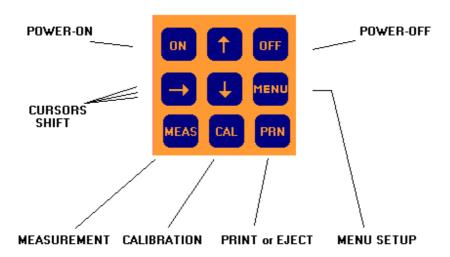
With the keys **ON** and **OFF** the power is applied to the instrument. After the power is switched on, the display shows
